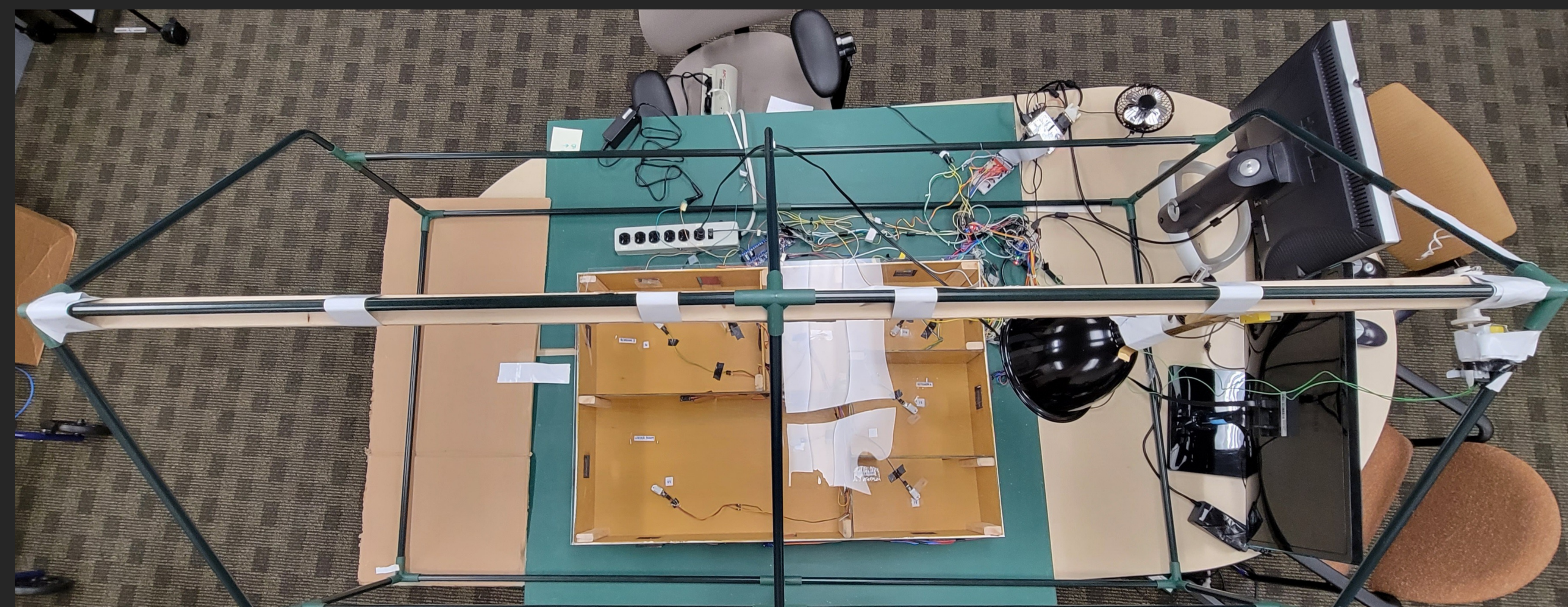
Figure 1: Experimental setup of ScaledHome, confined within the greenhouse. The motor controlling the Sun position is located on the right side of the picture, while the motor controlling the Sun tilt is on the suspended system itself.
