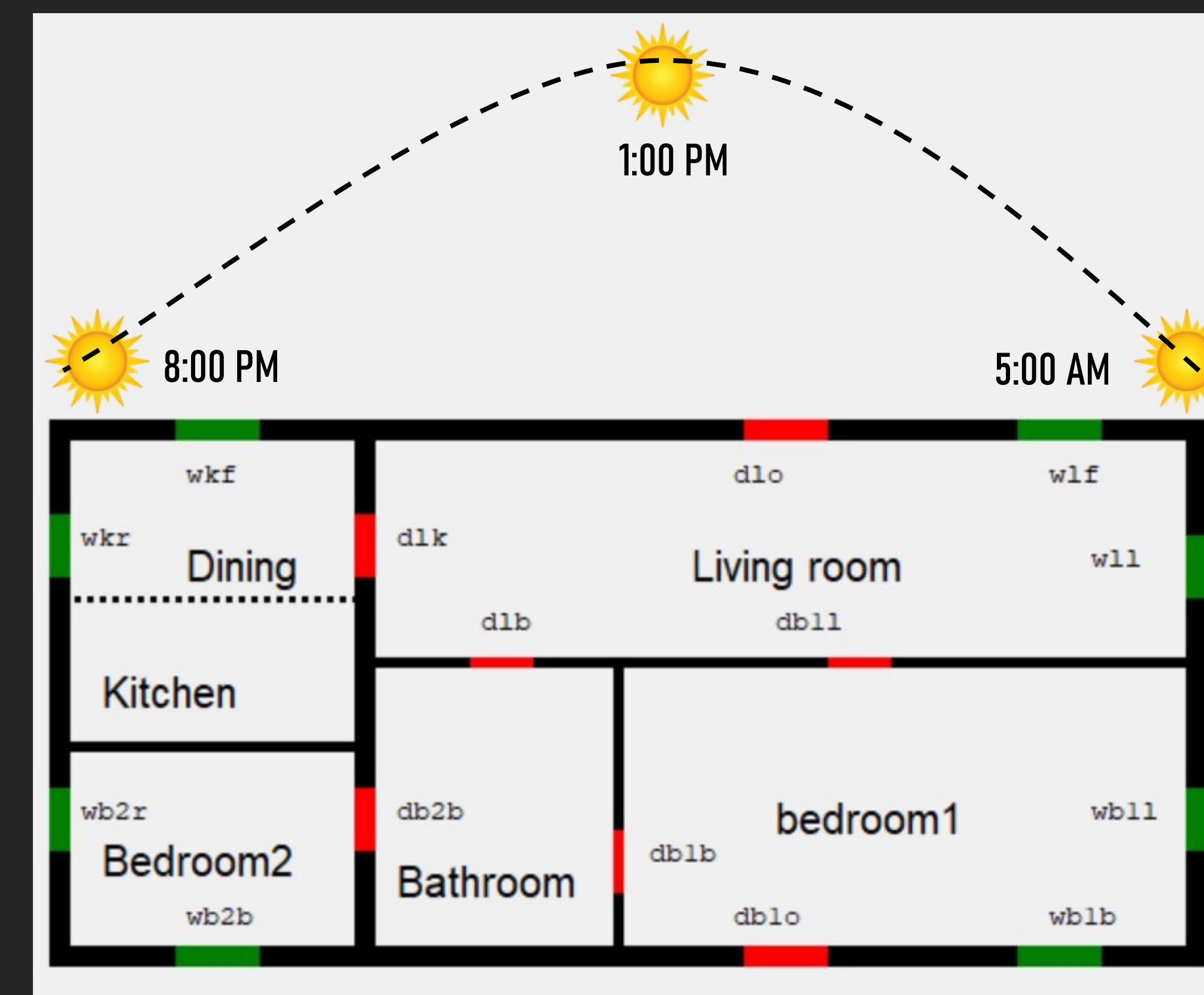
Figure 3: Virtual emulation of ScaledHome. The doors are labeled red while windows are labeled green. The sun moves from right to left.
