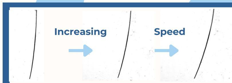
Figure 5: Fur motion and curvature in order (a) 10 mm coyote fur curved due to 546 mL/min flow rate, (b) 10 mm coyote fur curved due to 1300 mL/min flow rate, and finally, (c) 10 mm coyote fur curved due to 1896 mL/min flow rate
