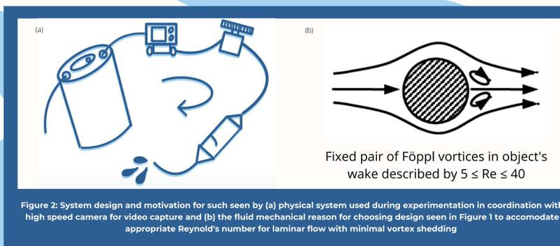
Figure 2: System design and motivation for such seen by (a) physical system used during experimentation in coordination with high speed camera for video capture and (b) the fluid mechanical reason for choosing design seen in Figure 1 to accommodate appropriate Reynold's number for laminar flow with minimal vortex shedding
