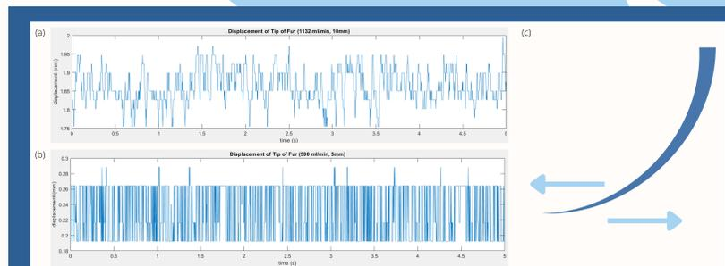
Figure 4: Fur motion described by (a) plot of displacement v. time of 10 mm coyote fur at flow rate 1132ml/min, (b) plot of displacement v. time of 5 mm coyote fur at flow rate 500ml/min and (c) the motion of fur being described in each plot with a fixed end inside laminarizing flow cell
