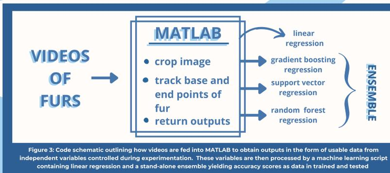
Figure 3: Code schematic outlining how videos are fed into MATLAB to obtain outputs in the form of usable data from independent variables controlled during experimentation. These variables are then processed by a machine learning script containing linear regression and a stand-alone ensemble yielding accuracy scores as data in trained and tested
