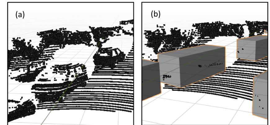
Figure 5. A sample from the KITTI dataset before (a) and after detection (b).
