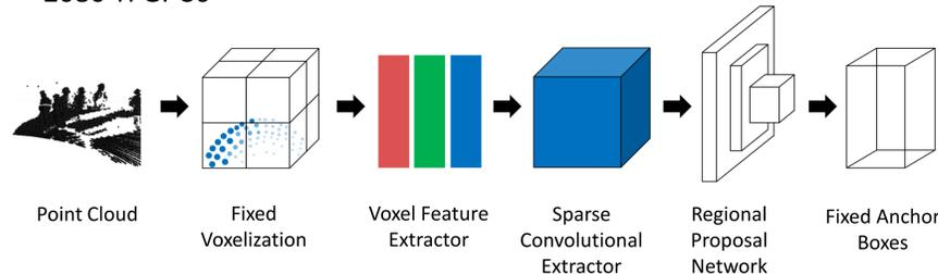
Figure 1. The SECOND (Sparsely Embedded Convolutional Detection) method pipeline used in experimentation as proposed by [1].
