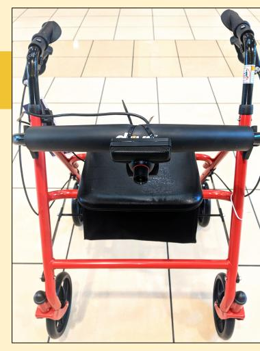
Figure 2. Walker with camera & RaspberryPi.
