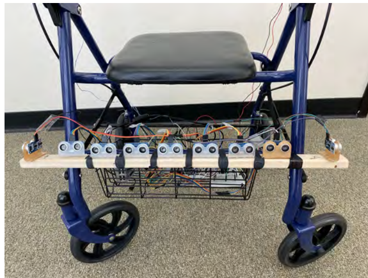
Figure 1. The rollator configured with nine HC-SR04 ultrasonic sensors. Seven sensors are facing forward to capture obstacles in a wide area in front of the walker. To facilitate navigational guidance, two sensors (one on the left and the other on the right) are capturing obstacles.
