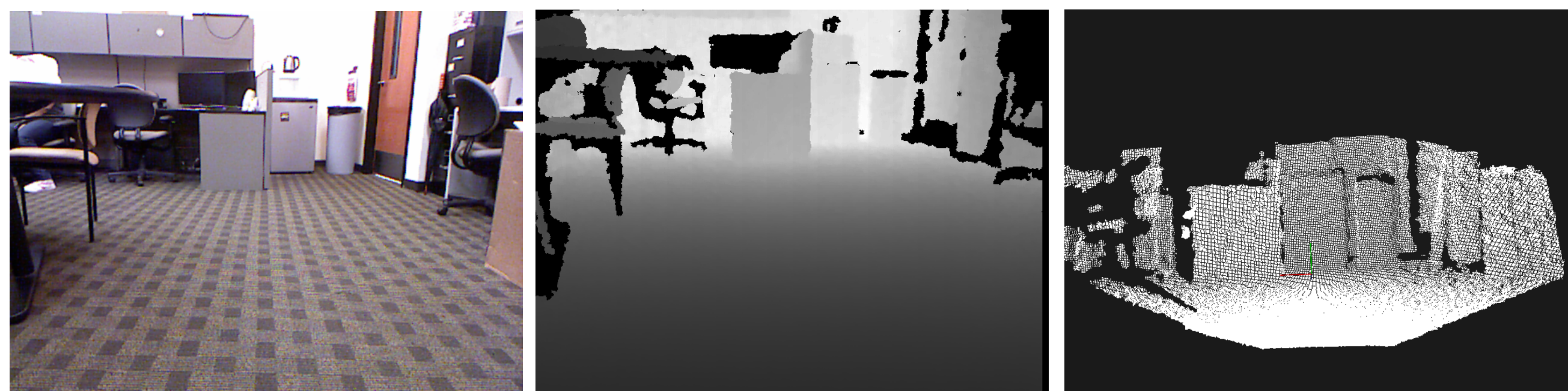
A scene captured in a color image, depth image, and point cloud (from left to right)
