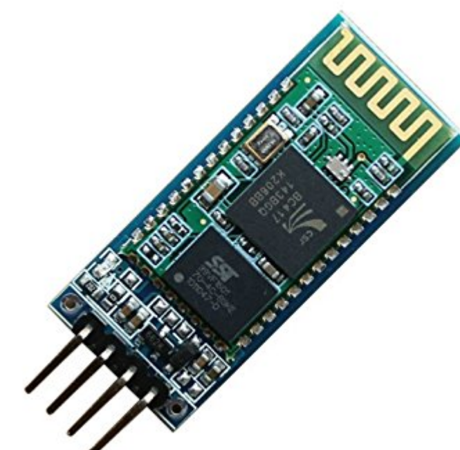
The HC-06 Bluetooth module used with the Arduino.
